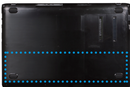
The location of the internal battery
